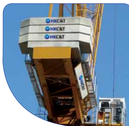
COUNT JIB & BALLAST BLOCK
